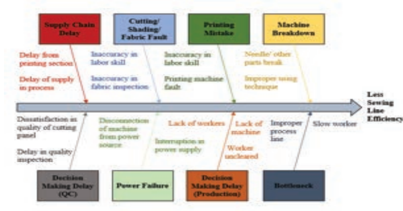
Figure 3. Cause-effect Diagram of Root Causes of Less Efficiency in Sewing Section .
