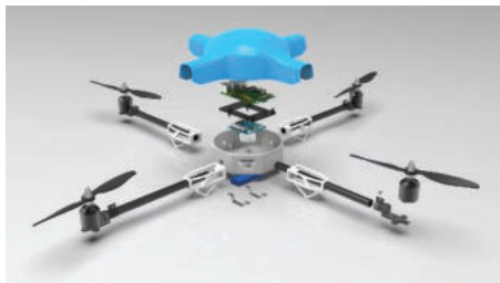
Figure 2. Conceptual CAD model of the quadcopter .
